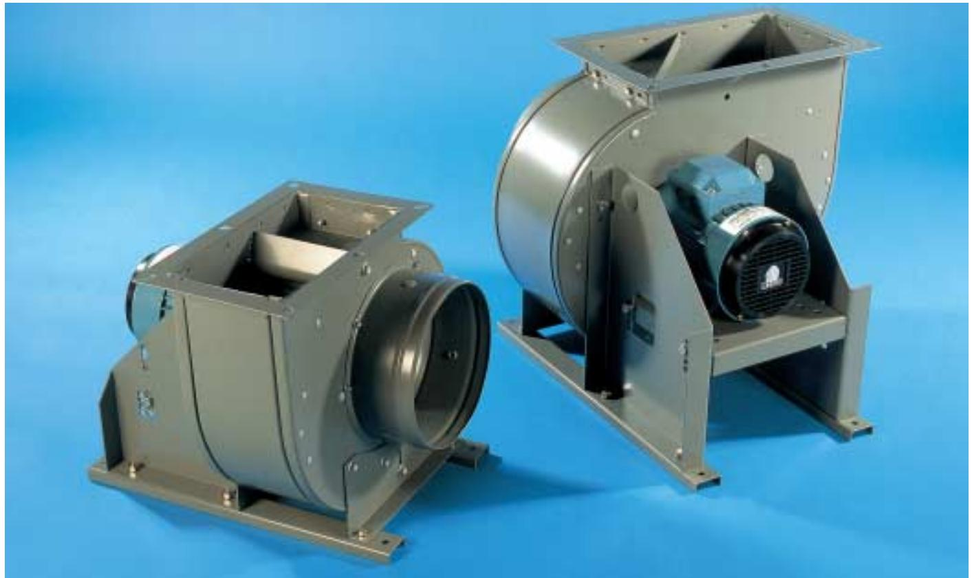
The type GT CENTRIMASTER direct driven, single-inlet centrifugal fans cover air flows up to  $7 \text{ m}^3/\text{s}$  and pressure rises up to 2.000 Pa. The fan series consists of centrifugal fans available with two types of impeller:
