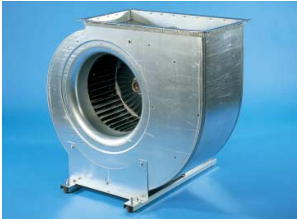
Single-inlet centrifugal fan for a direct-drive. The fan casing is made of Sendzimir galvanised sheet steel, jointed by the "Pittsburg folding method". Fan impeller with forward-curved blades, made of Sendzimir galvanised sheet steel. The fan impeller is dynamically balanced to accuracy according to ISO Standard 1940 – 1973 G 6.3.
