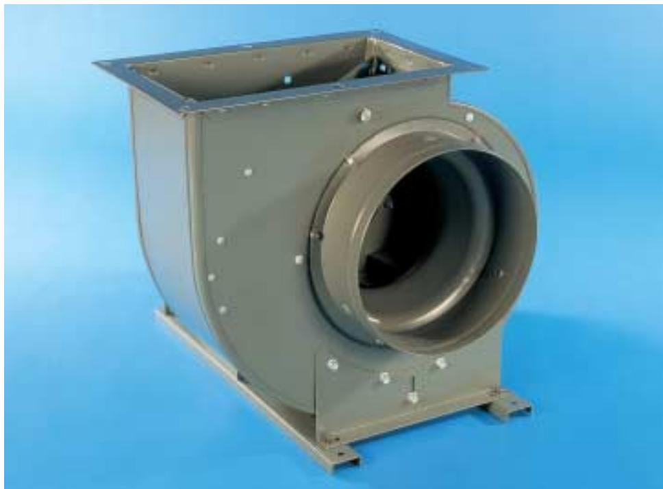
Single-inlet centrifugal fan for a direct-drive. The fan casing is made of Sendzimir galvanised sheet steel, jointed by the "Pittsburg folding method". Fan impeller with backward-curved blades, made of sheet steel, welded and coated with 60 mm thick epoxy powder. The fan impeller is dynamically balanced to accuracy according to ISO Standard 1940 – 1973 G 2.5 (sizes 035–071) or G 6.3 (sizes 022–031).
